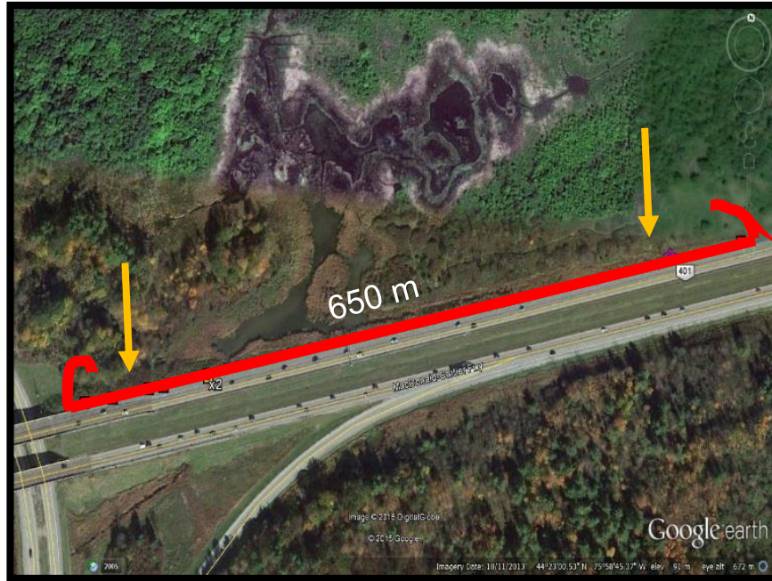
Figure 27. Proposed mitigation fence location (red) and nesting beach habitat (orange arrows) to prevent target SAR turtles from entering the road at Hotspot I.
